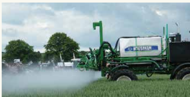
Nozzles operating at too high a pressure – unacceptable drift
