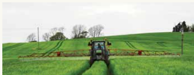
Boom at 50cm – the correct height
